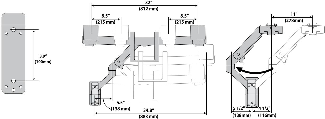
**EN** Top view showing range of motion when pulled out from the wall.
