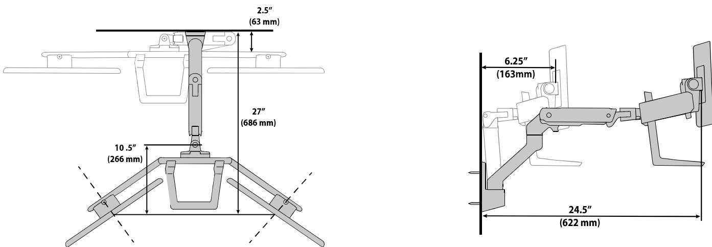
**EN** NOTE: Determine if arm will typically collapse to the left or right before installation.
