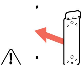
**EN** CAUTION: Make sure the wall mount bracket is level, flush and snug to the wall surface. DO NOT OVERTIGHTEN THE BOLTS.
