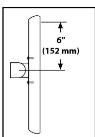
**[EN]** Mounting height assumes there is a 6" (152 mm) distance between the center of your monitor mounting holes and the top of the screen. If your distance is smaller, you should increase mounting height accordingly; if your distance is larger, you should decrease your mounting height accordingly.
